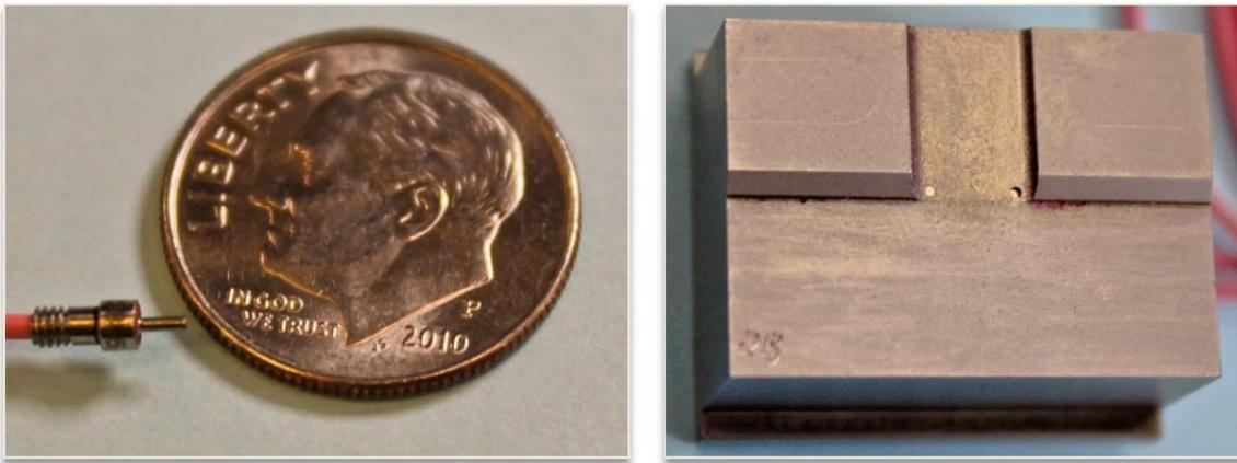
*Temperature sensor (L) and two sensors mounted in a cavity block (R)*
